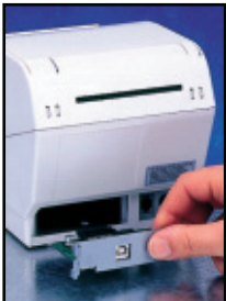
High speed USB and Ethernet interface options (user installable)
